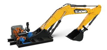
With main body adopting H-beam rigid structure, the whole machine's strength is reinforced, and the turntable side fream adopts the D-tube structure to improve its ability to resist external impact.
